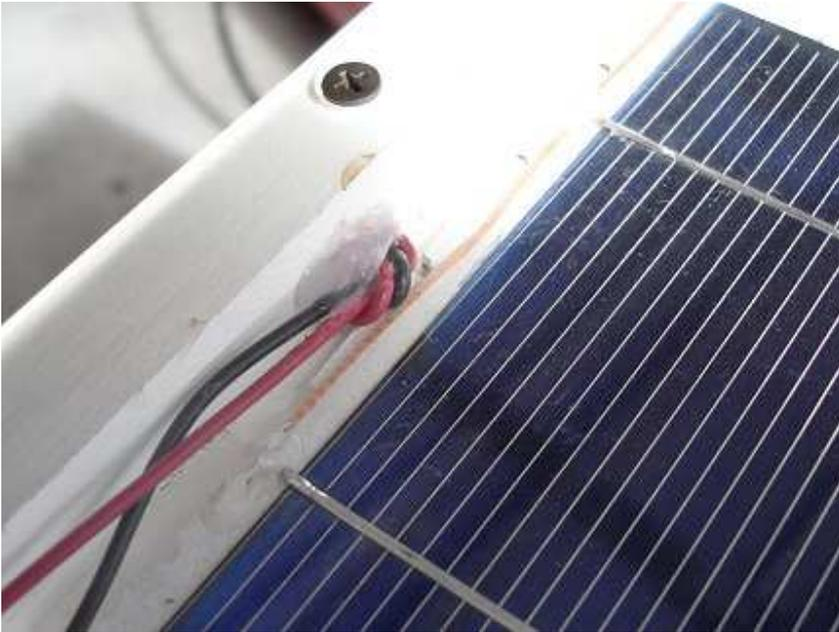
I drilled a hole in the back of the panel near the top for the wires to exit. I put a knot in the wires for strain relief, and anchored them in place with yet more of the silicone caulk.
