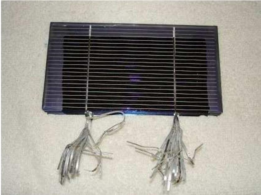
I bought a couple of bricks of 3 X 6 mono-crystalline solar cells. It takes a total of 36 of these type solar cells wired in series to make a panel. Each cell produces about 1/2 Volt. 36 in series would give about 18 volts which would be good for charging 12
