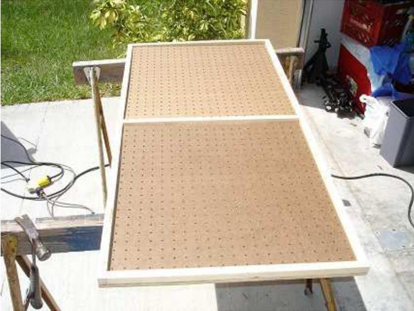
Next I cut two pieces of masonite peg-board to fit inside the wells. These pieces of peg-board will be the substrates that each sub-panel will be built on. They were cut to be a loose fit in the wells. You don't have to use peg-board for this. I just
