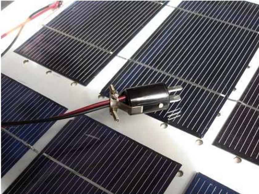
I added a polarized two-pin jones plug to the end of the panel wires. A mating female plug will be wired into the charge controller I use with my [home-built wind turbine](#) so the solar panel can supplement it's power production and battery charging
