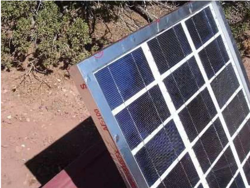
Here is a close-up of the solar panel after having the edges sealed with aluminum tape. This is not the cheap duct tape. This is the thin metal tape with an adhesive backing. I applied it all the way around the edges of the panel and across
