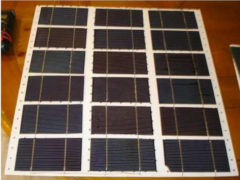
Next time I will do it differently. I will solder tabs onto the backs of all the solar cells. Then I will glue all the cells down in their proper places. Then I will solder the tabs together. It seems like the obvious way to go to me now, but I had to do it the hard way
