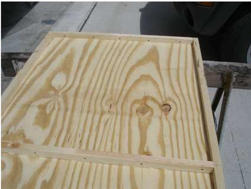
Here is a close-up showing one half of the main panel. This well will hold one 18 cell sub-panel. Notice the little holes drilled in the edges of the well. This will be the bottom of the panel (it is upside down in the photo, sorry). These are vent holes to keep the
