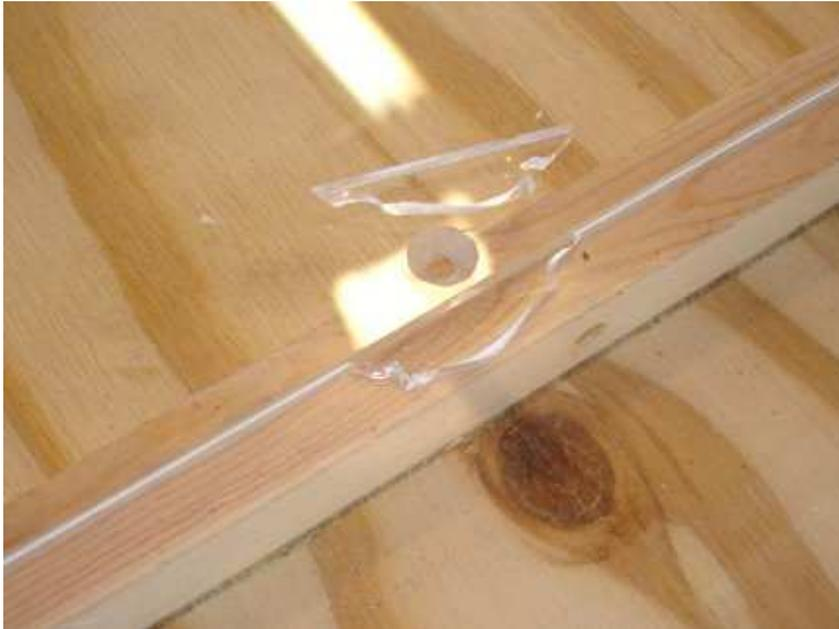
Oops! This photo shows a close-up of where the two halves of the plexiglass cover meet over the center divider. I drilled and countersunk holes all around the edges of both pieces of plexiglass so I could screw them onto the face of the panel
