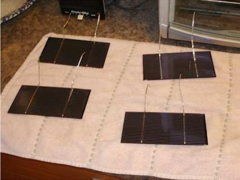
Here are some separated and cleaned solar cells drying on a towel. Once separated from their wax stabilized brick form, they are amazingly fragile and difficult to handle and store. I would recommend leaving them as bricks until you
