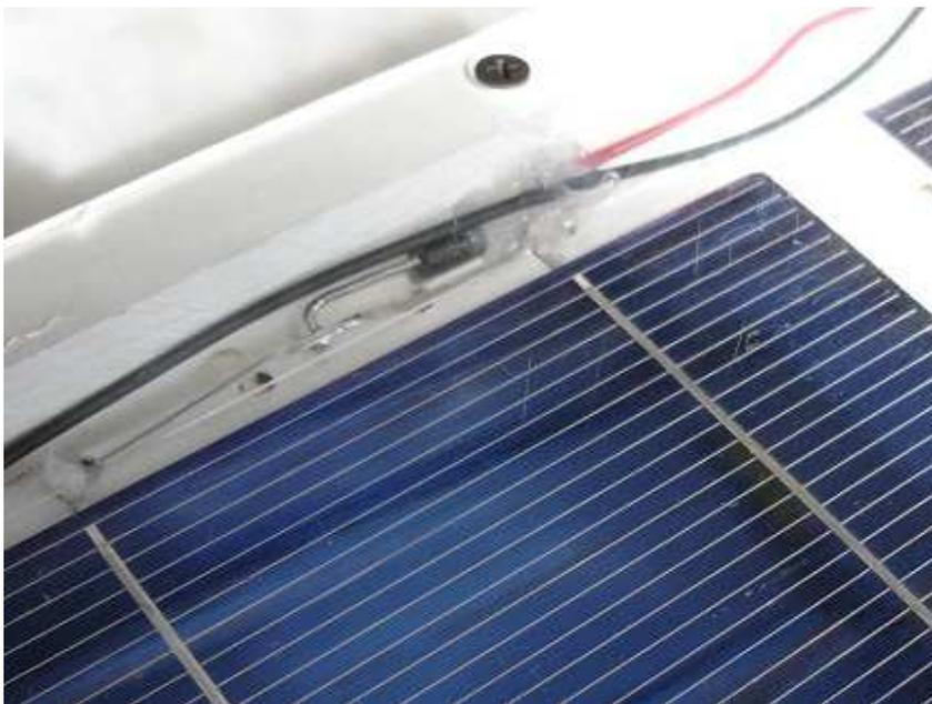
Each solar panel in a solar power system needs a blocking diode in series with it to prevent the panel from discharging your batteries at night or during cloudy weather. I used a Schottky diode with a 3.3 Amp current rating. Schottky diodes have a much
