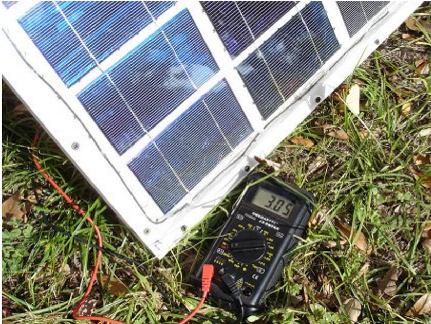
Here I am testing the current capacity of the panel, again in bright winter sunlight. My meter says 3.05 Amps short circuit current. That is right about what the cells are rated for. So the panel is working very well.
