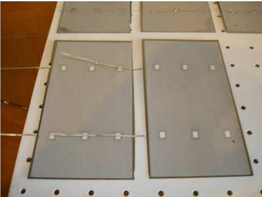
I started out by drawing a grid pattern on each of the two pieces of pegboard, lightly in pencil, so I would know where each of the 18 cells on them would be located. Then I laid out the cells on that grid pattern upside-down so I could solder them
