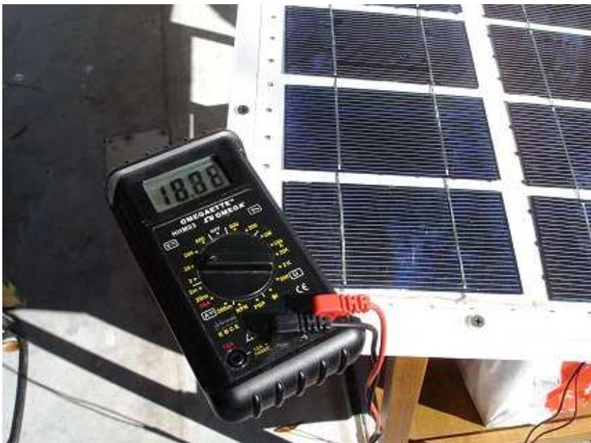
Here I am testing the Voltage output of the completed panel in bright winter sunlight. My meter says 18.88 Volts with no load. That's exactly what I was aiming for.
