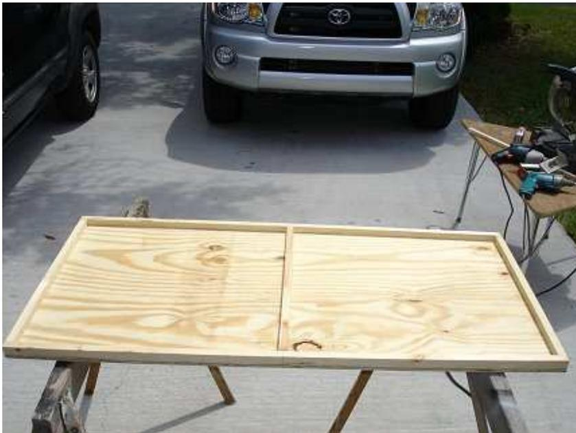
A solar panel is really just a shallow box. So I started out by building myself a shallow box. I made the box shallow so the sides wouldn't shade the solar cells when the sun comes at an angle from the sides.
