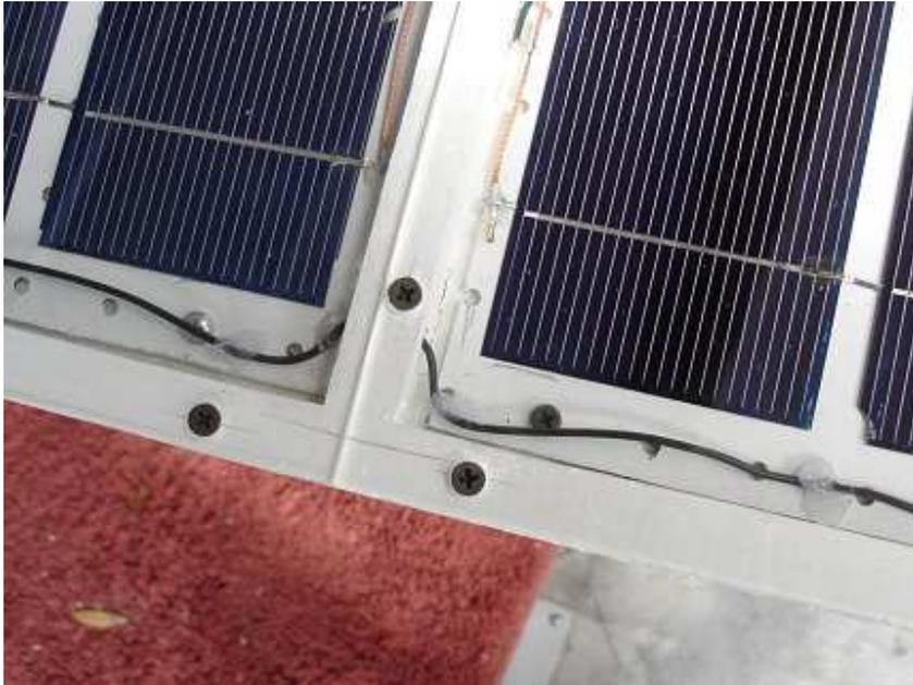
Wires to connect the two half panels together were run through the vent holes in the central divider. Again, blobs of silicone caulk were used to anchor the wire in place and prevent it from flopping around.
